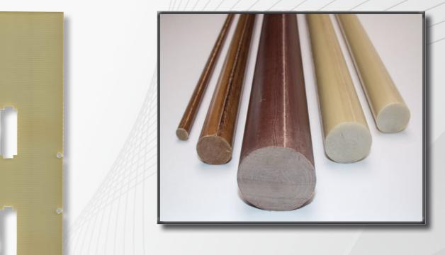
Laminated moulded tubes and rods are manufactured in moulds by rolling epoxide or phenolic impregnated layers of material on mandrel and curing at high temperature and under preassure.
